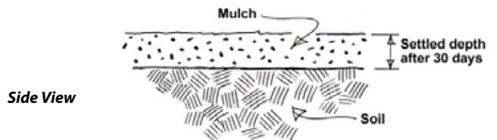
About 30 days after spreading, the mulch should have naturally settled by the settlement depth shown at right, to give the minimum desired settled depth.
